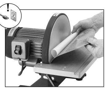
**Figure 5.** Sandpaper being slipped between the disc and table.
